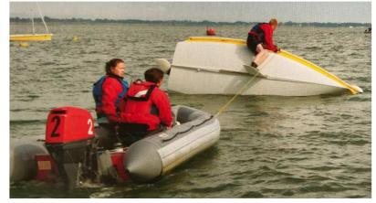
RIB tow method. A line is secured to the bow of the dinghy
